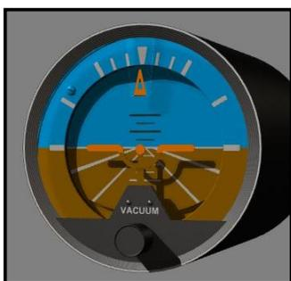
The artificial horizon gauge is essential when flying in the dark or in clouds. Basically, it tells you where up is and shows you how to keep the airplane balanced.
